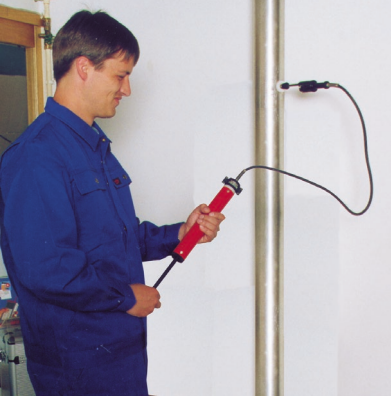
Fig. 4: Extracting the smoke gas
