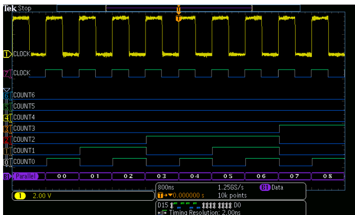
The MDO3000 with MDO3MSO option provides 16 integrated digital channels enabling you to view and analyze time-correlated analog and digital signals.
