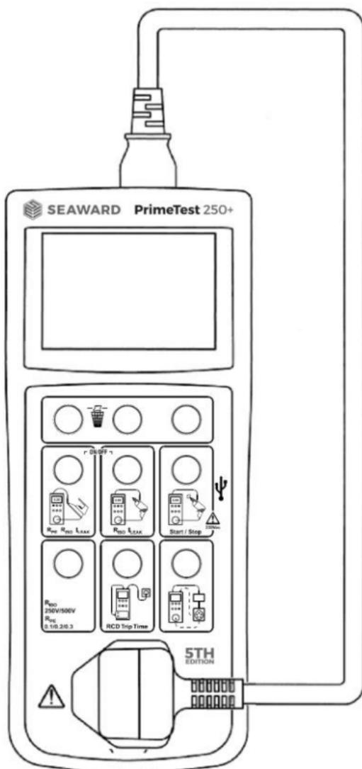
Figure 7. Testing IEC Leads
