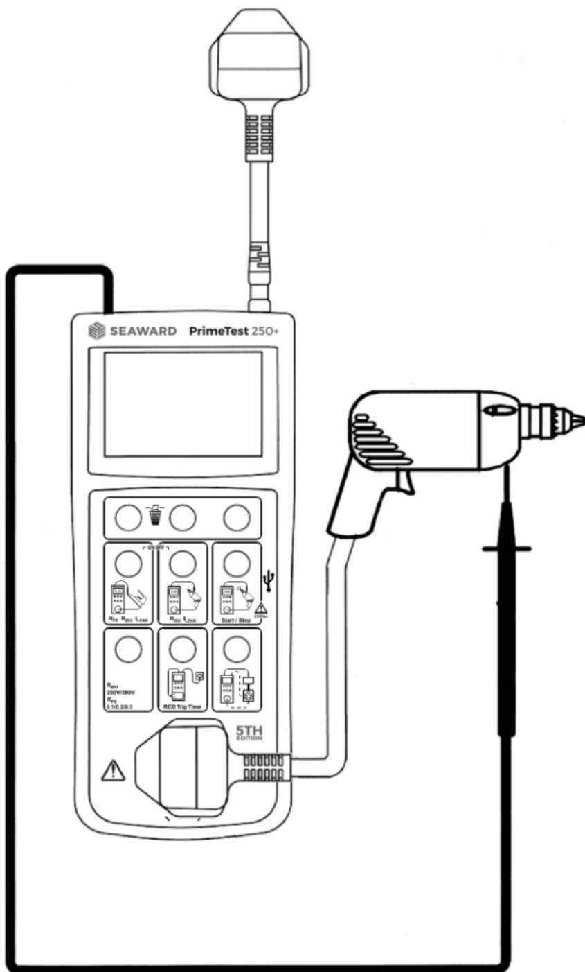
Figure 5. Testing CLI appliances, mains leakage
