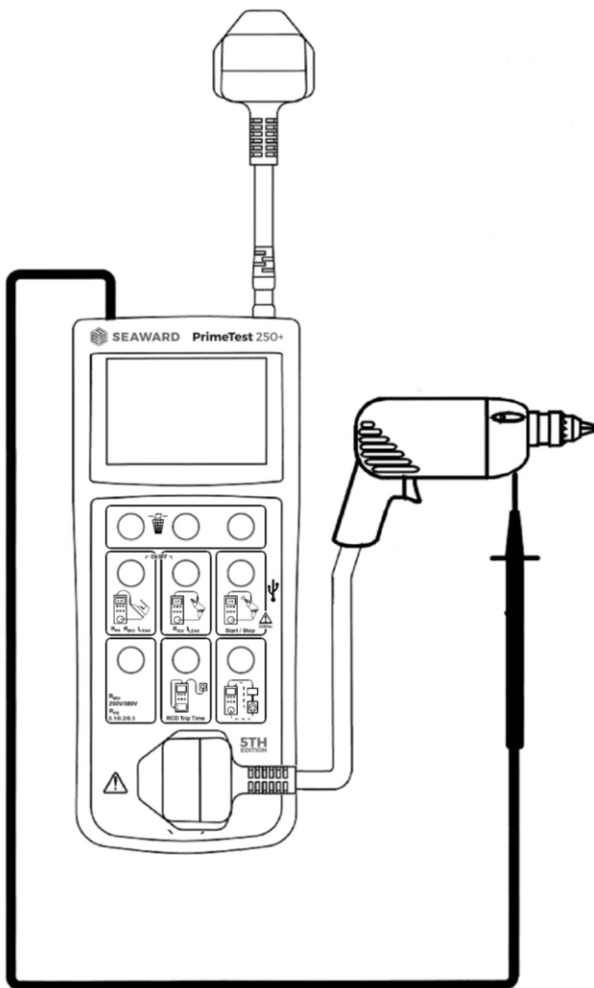
Figure 6. Testing CLII appliances, mains leakage
