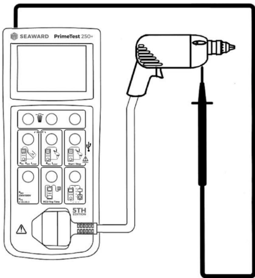
Figure 4. Testing CLII appliances, no mains leakage
