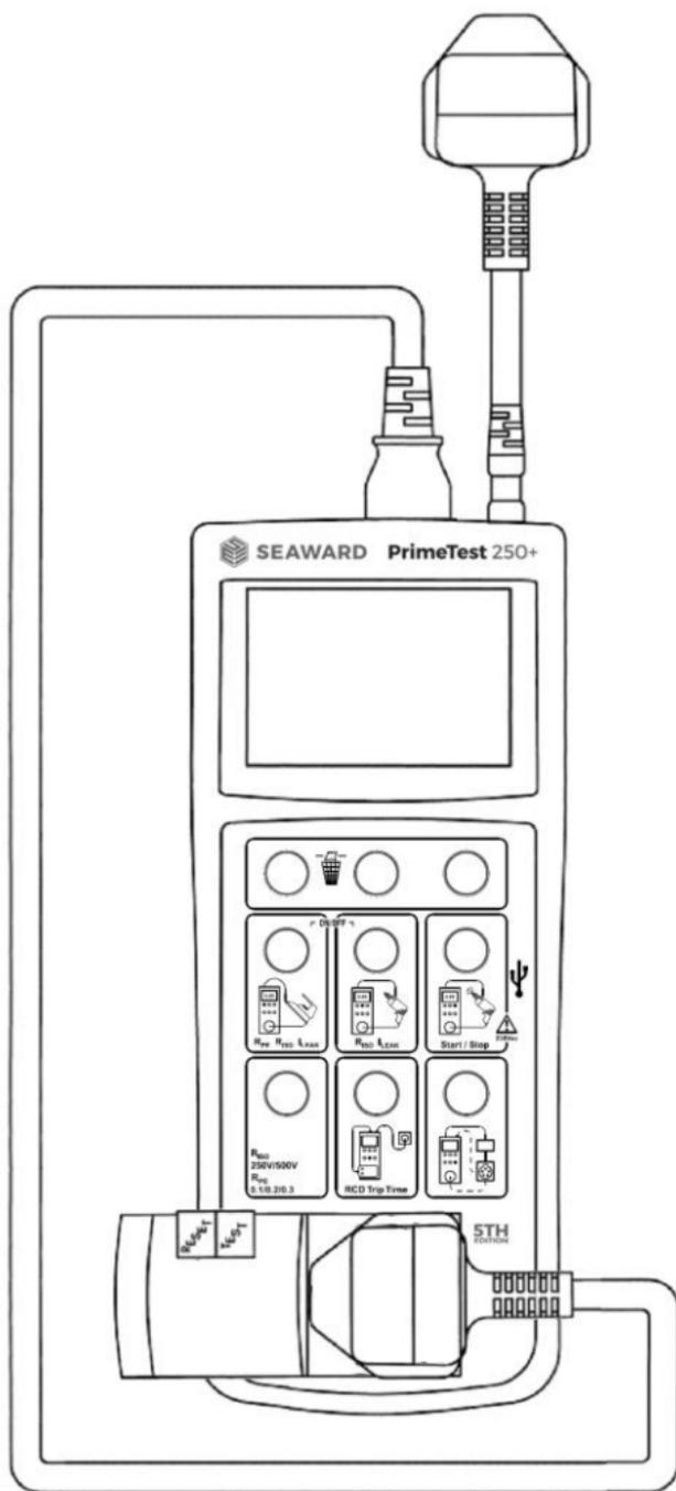
Figure 9. Testing Plug Top RCD
