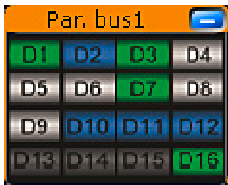
The signal activity of the digital channels is displayed in the signal icon independently of the oscilloscope settings.
