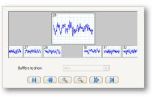
scope. Combined with mask limit testing, the buffer navigator can be instructed to show only waveforms that are out of specification.
