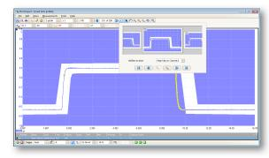
The numerical and graphical mask editors can be used separately or in combination, allowing you to enter accurate mask specifications and to modify existing masks. You can import and export masks as files.
