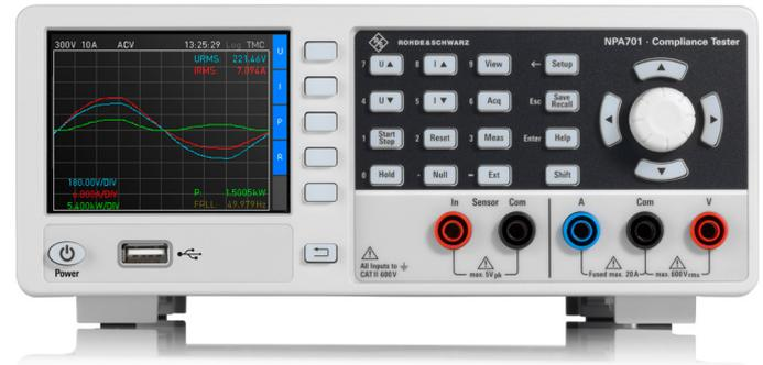
The instrument has wizards for the IEC 62301 (standby), EN 50564 (extended standby) and EN 61000-3-2 (harmonic current for EMC, CE approval) standards, enabling autonomous measurements without a PC.
