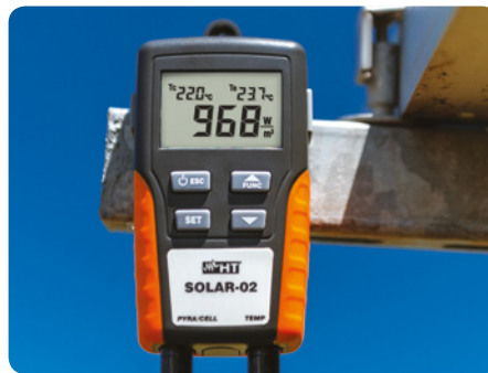
Solar02 remote unit.
