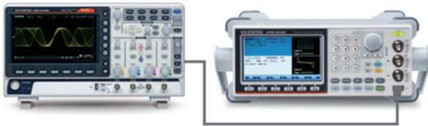
Direct Waveform Reconstruction from the DSO
