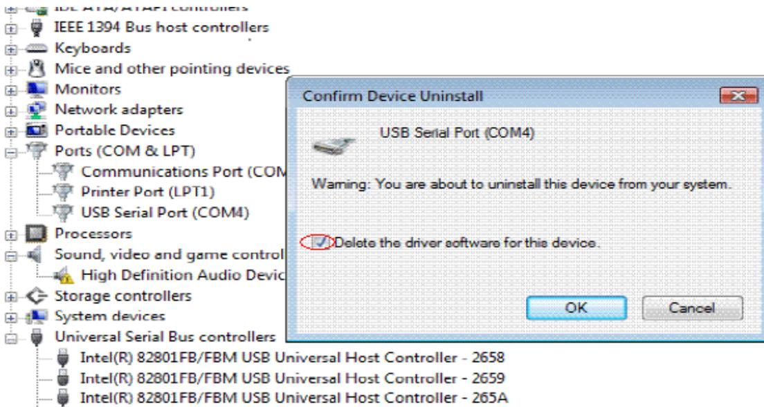
**Note:** if you have more than one USB Serial Port (COMx) installed in your PC, you need to repeat from step 5 to step 6 to delete the driver software for each port.
