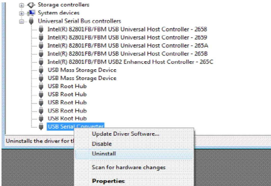
8. Select uninstall and be sure to click the box for “Delete the driver software for this device” in the next window and press “OK”.
