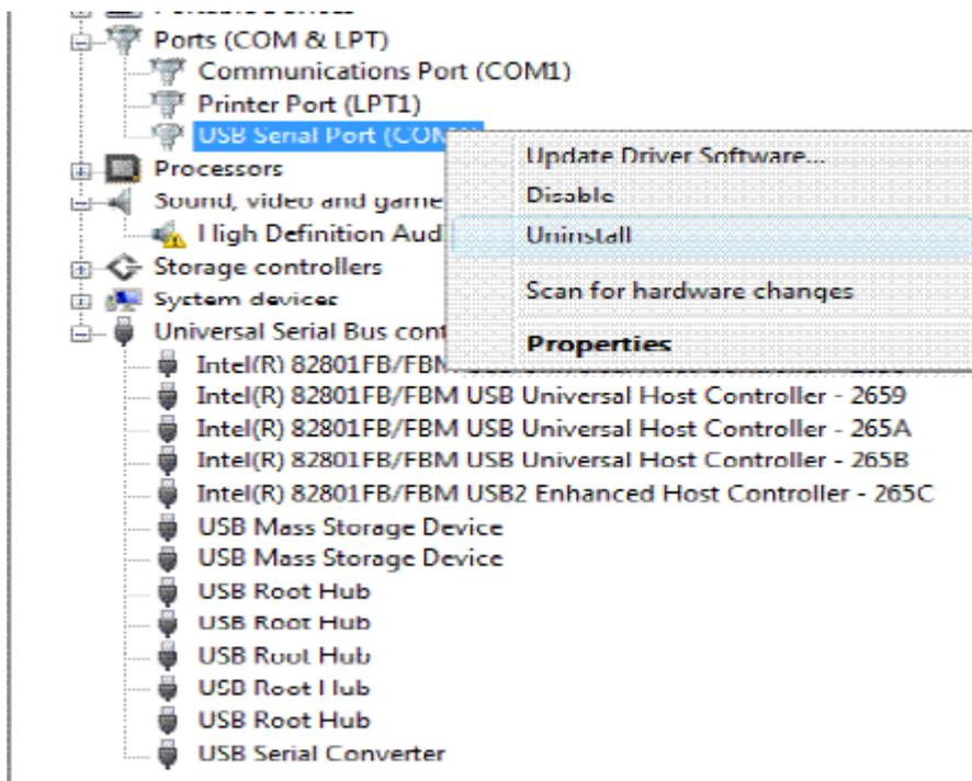
6. Select uninstall and be sure to click the box for “Delete the driver software for this device” in the next window and press “OK”.
