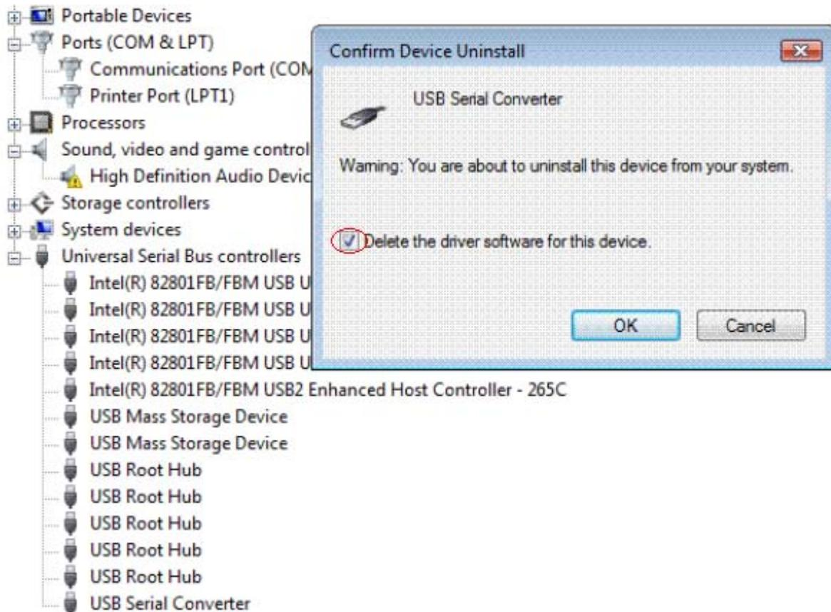
**Note: if you have more than one USB Serial Converter installed in your PC, you need to repeat step 7 and step 8 to delete the driver software for all devices.**
