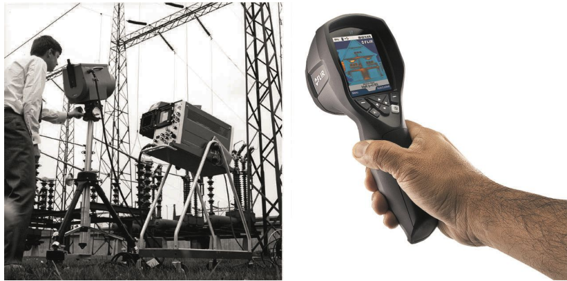
Figure 11.2 LEFT: Thermovision Model 661 from 1969. The camera weighed approximately 25 kg (55 lb.), the oscilloscope 20 kg (44 lb.), and the tripod 15 kg (33 lb.). The operator also needed a 220 VAC generator set, and a 10 L (2.6 US gallon) jar with liquid nitrogen. To the left of the oscilloscope the Polaroid attachment (6 kg/13 lb.) can be seen. RIGHT: Flir i7 from 2012. Weight: 0.34 kg (0.75 lb.), including the battery.
