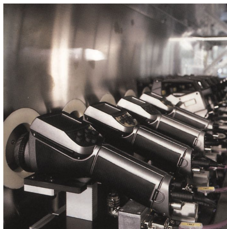
Figure 11.5 LEFT: Testing of infrared cameras in the climatic chamber; RIGHT: Robot used for camera testing and calibration
