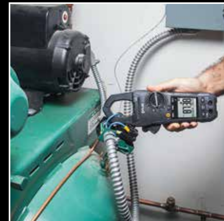
Inrush Current detects start-up current spikes
