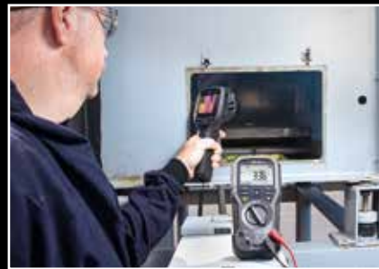
Use METERLiNK to embed electrical readings into FLIR IR camera images
