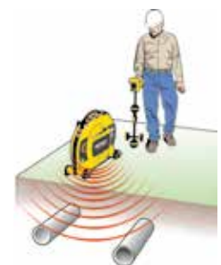
Induce a signal to locate utilities.
