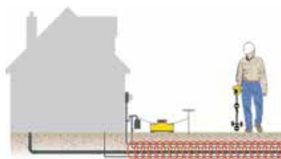
Direct connect to utility lines.
