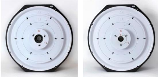
Flow ring D attaches directly to the center of ring B (remove ring C before inserting ring D). The letter D faces upward. When using flow ring D or E, the red tubing for measuring the flow of the fan (fan pressure) connects to ring D.
