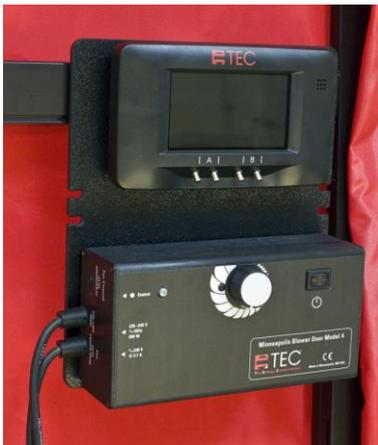
Hang the fan speed controller and the DG-1000 on the upper of the two cross bars using the clamp on the back of the gauge board. Before connecting the speed controller to the fan, make sure the switch on the controller is set to “off” and that the control knob is turned completely to the left (minimum).
