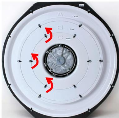
To **change the flow ring**, rotate the ring clips to remove a flow ring. Insert the correct ring face-up (identifying letter facing up and the flow nozzle pointing into the fan) and retighten the fastener clips.
