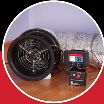
The **Minneapolis Duct Blaster**<sup>®</sup> is used to measure the airtightness of ductwork.
