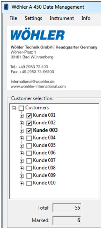
Fig. 13: Mark all customer files to be transmitted
