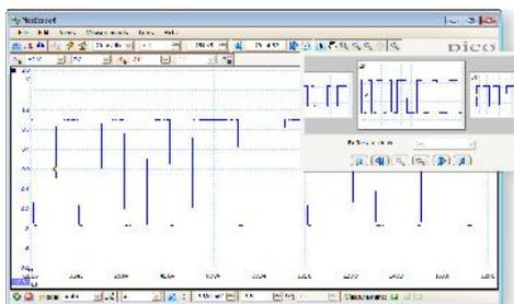
To help you find your way around the buffer memory, you can divide it into as many as 10,000 individually triggered segments. Use the visual buffer navigator to scan through the segments, or set up a mask to filter out the waveforms of interest.
