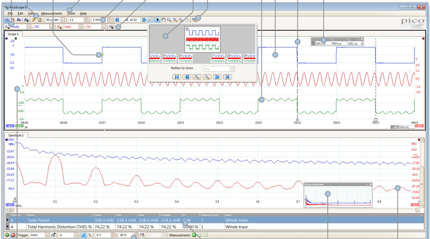
**Movable axes:** The vertical axes can be dragged up and down. This feature is particularly useful when one waveform is obscuring another. There's also an **Auto Arrange Axes** command.
