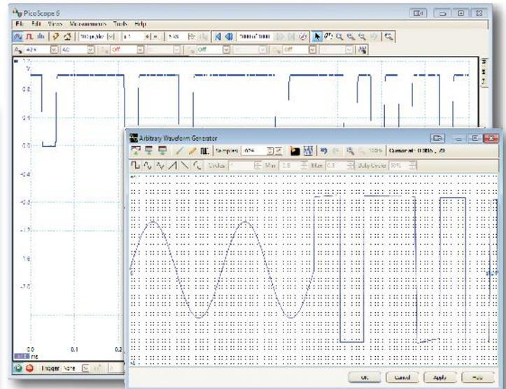
Every model includes a built-in DC to 20 MHz function generator with sine, square, triangle and DC waveforms. D models add a built-in 12-bit, 200 MS/s arbitrary waveform generator. You can import arbitrary waveforms from data files or create and modify them using the built-in graphical AWG editor.
