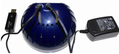
Fig. 6: Dorsal view of the device: Connection of the power supply block and the USB cable
