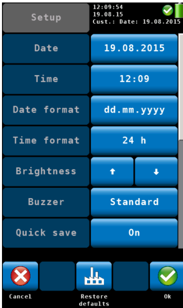
Fig. 61: Setup menu, the scroll bar shows that there are more parameters available.
