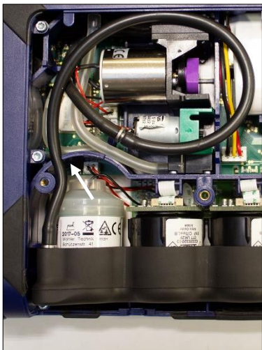
Fig. 75: Connecting tube, correctly positioned, guiding hooks marked by an arrow.
