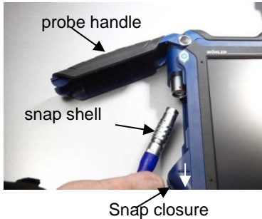
Fig. 27: Wohler A 550 INDUSTRIAL with open probe compartment
