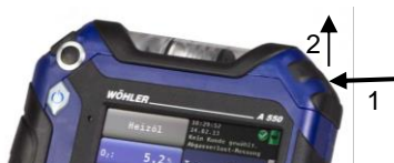
Fig. 67: Open the condensate trap compartment
