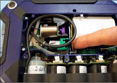
Fig. 76: Pulling out the battery plug
