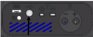
Fig. 45: Connectors for the wood moisture probe at the bottom of the analyzer
