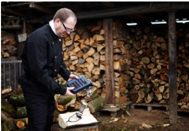
Fig. 46: Wood moisture measurement with Probe Wohler HBF 420.
