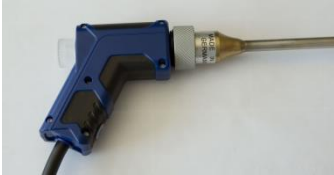
Fig. 26: Probe handle with gas probe 1,000 mm
