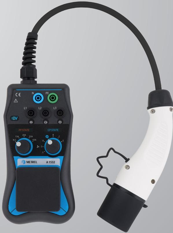
The A 1532 EVSE adapter is a special accessory intended for testing Electric Vehicle Supply Equipment (EVSE) together with supported METREL installation testers. It is used for verification of electrical safety and functional testing of EVSE. It is intended for testing Mode 3 EV supply equipment with a type 2 connector.
