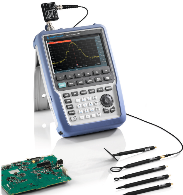
The R&S® Spectrum Rider with near-field probes and DUT.
