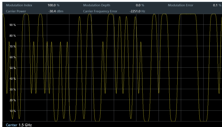
Figure 17-4: Modulation depth of a 2ASK signal
