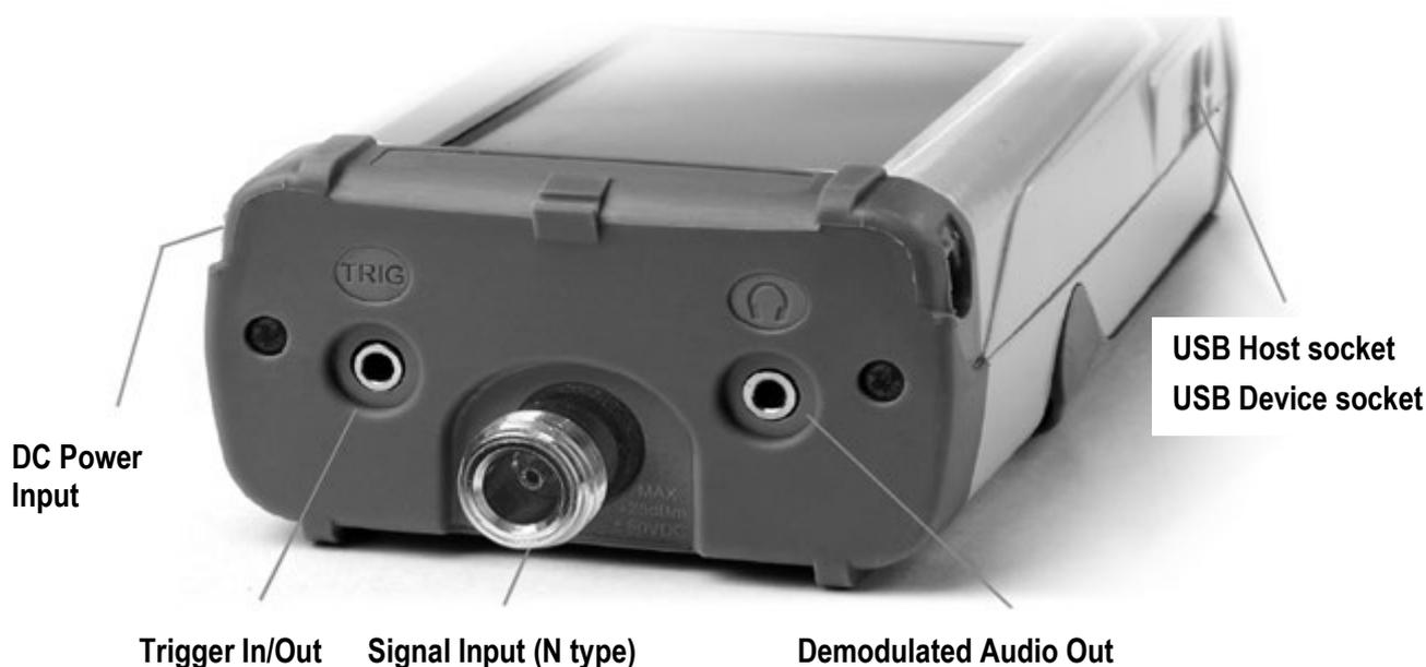
**DC Power Input** 1.3mm power socket mounted on the right hand side of the instrument.
