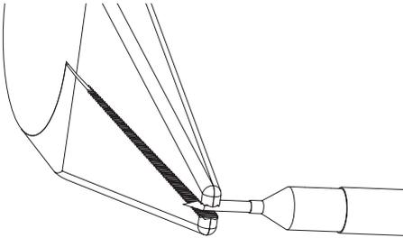
Use pliers to grip and pull the probe carefully out of its contact socket.
