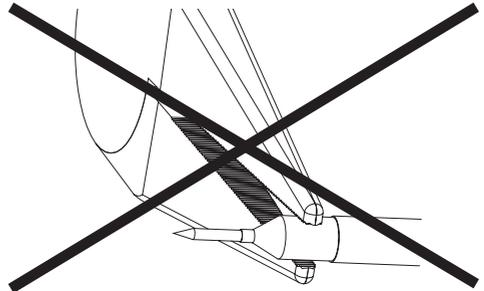
Do not grip the white plastic insulator or the probe housing with pliers.
