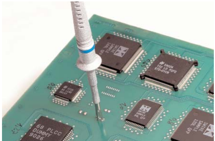
"Hands-free-probing" with PCB Adapter
