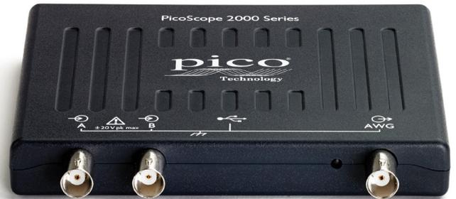
2-channel oscilloscope: 2206B, 2207B and 2208B
