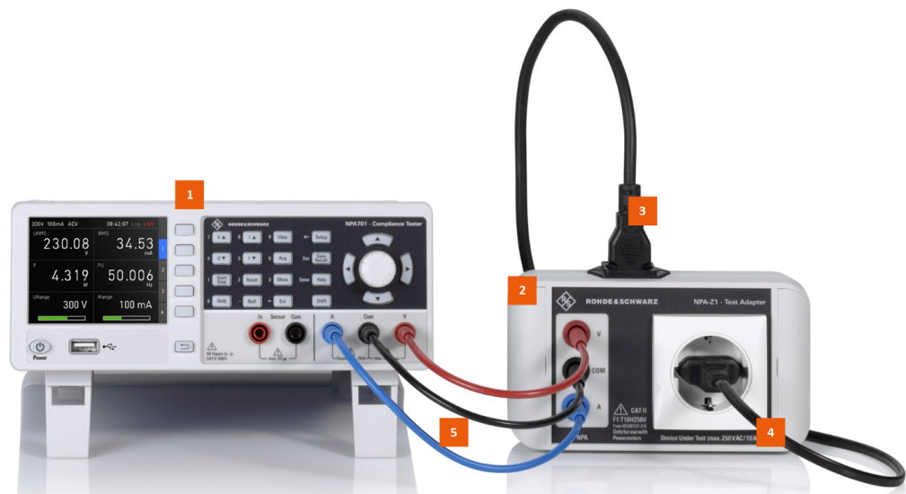
Figure 3-3: Measurement setup of the R&S NPA and the R&S NPA-Zx to a DUT
