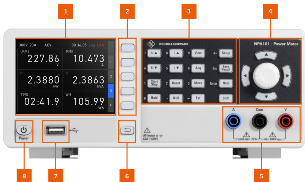
Figure 3-5: Front view of the R&S NPA101
