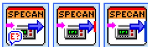
Fig. 4-9: Fast Write icons: with Error Checking / with OPC? synchronisation / with \*WAI synchronisation.
