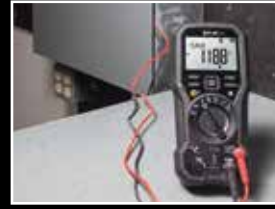
Use Automatic Data Recording to find intermittent errors
