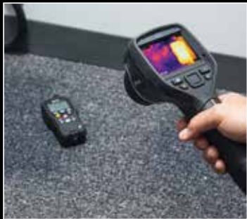
Use METERLiNK to embed moisture data into FLIR IR camera images
