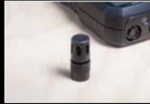
Temperature/humidity sensor is field replaceable
