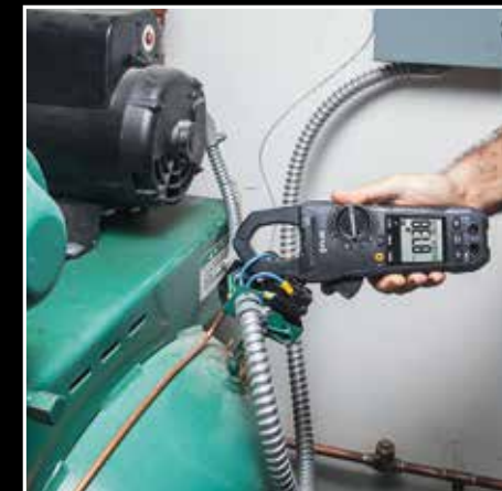
Inrush Current detects start-up current spikes
