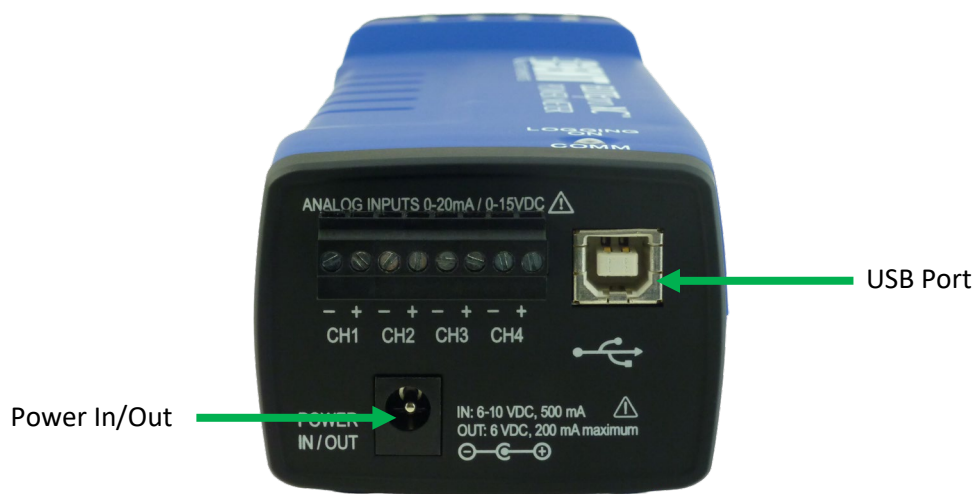
Power End Panel Connections
