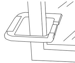
The device comes with an additional glass thickness gauge. The gauge enables measuring the thickness of monolithic glass panes of up to 25 mm. In case of insulated glazed units, only the accessible panes can be measured.
