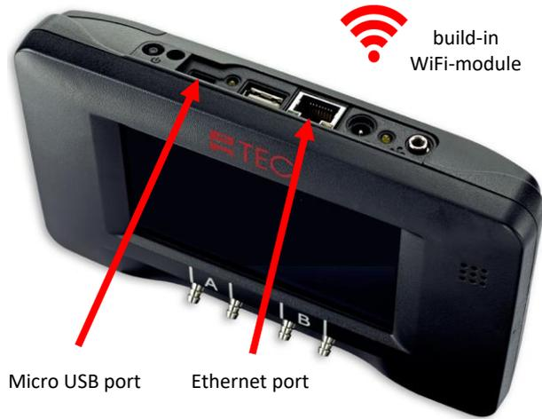
Fig. 2.1: DG-1000 communication ports
